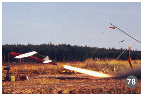
Picture78: Northrop BTT Radioplane, known in Finland as Male 82, being launched with a JATO rocket. (The Finnish Anti-Aircraft Museum)
