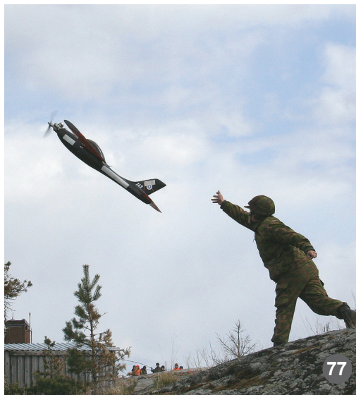
Picture 77: AA Male 97 target drone is hand launched. (The Finnish Anti-Aircraft Museum)
