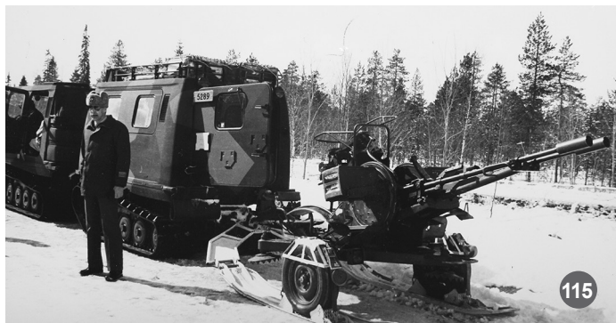
Picture 115: Increasing the mobility of AA units was tested over the snowy terrain of northern Finland in 1986. The commander of Rovaniemi AA battery, LtCol Ahti Lappi standing next to a 23mm AA gun equipped with skis. (The Finnish Anti-Aircraft Museum)
