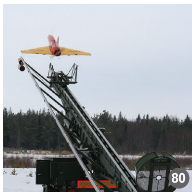
Picture 80: Meggitt Banshee target drone has been launched from a catapult. (The Finnish Defence Forces)
