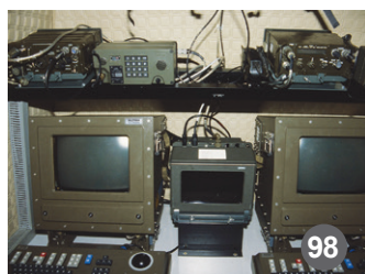
Picture 100: Tuliasemapääte (TASP) was a touch screen device designed by NOKIA. (The Helsinki Anti-Aircraft Regiment archives)
